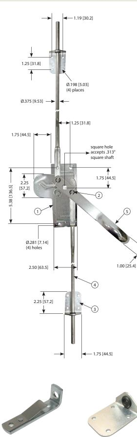
Spring Loaded Rod Guide part no. 718-01
