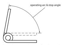
$inside\ stop\ hinges\ normally\ operate\ from\ the\ 0^\circ\ or\ closed\ position,\ stopping\ at\ a\ specific\ angle\ plus\ or\ minus\ 3^\circ.$
