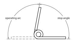
**outside stop** hinges normally operate from the 180° or flat, open position, stopping at a specific angle plus or minus 3°.
