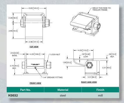
Pair of H3032 tilt hinges are suitable for use on trailers with GVWR rating up to **32,000lbs**
