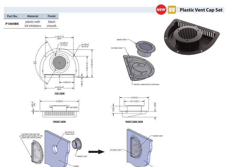
INSTALL OUTSIDE VENT TO THE OUTSIDE OF THE PANEL WITH (6) SCREWS (NOT SUPPLIED).
