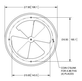
DRILL 3" [76mm] HOLE THROUGH THE PANEL AS SHOWN.
